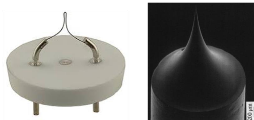
Figure 3. Different types of EM emitters: thermal emission (left) and field emission (right).
